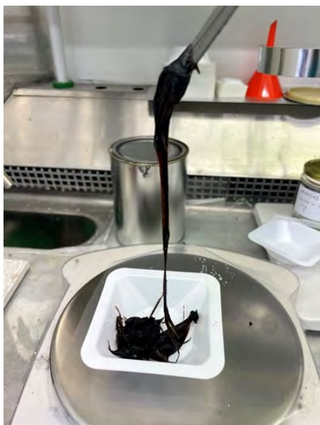
Figure 26. Lignin-PEI coatings on metal, showing the set-up for adhesion testing.
