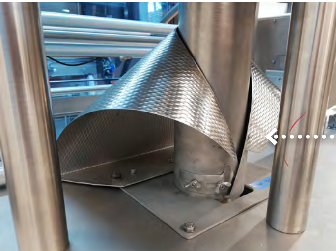
Figure 35. VFFS equipment used in the study, including a close-up of a forming shoulder.
