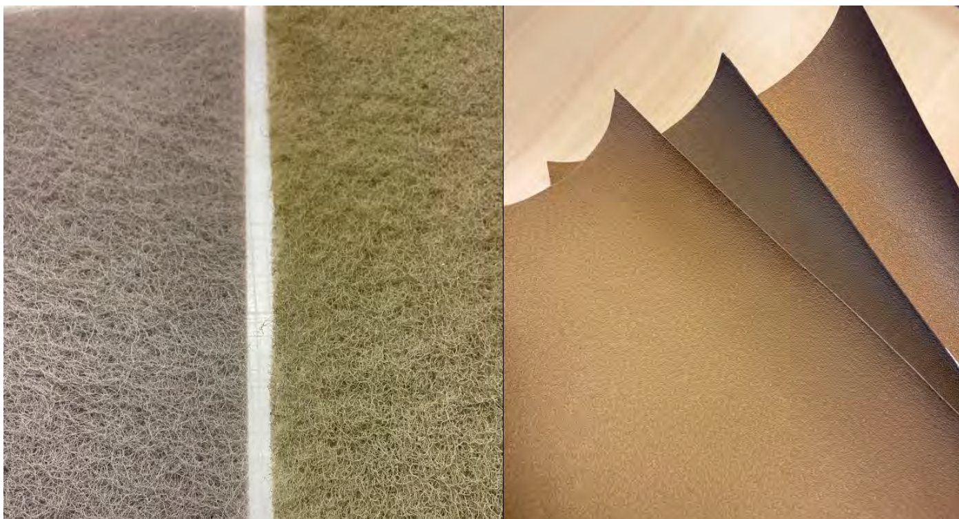
Figure 30. Spray- and roll-coated nonwoven and paper abrasives with lignin coatings
