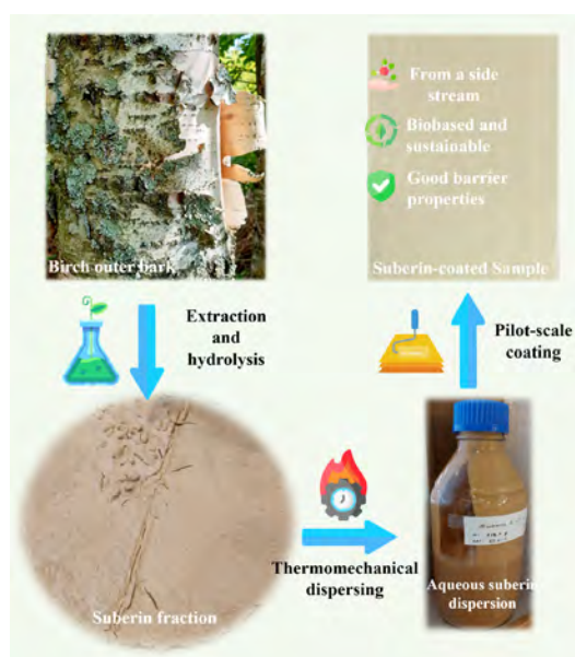
Figure 14. (left side) Overview of suberin isolation from birch bark and formation of aqueous suberin dispersions for barrier coatings for paper and paperboard substrates. (Right side) Water vapour transmission rate (WVTR) of coated paperboard samples in different coating conditions, 23 °C/50% RH, 23 °C/80% RH and 38 °C/90% RH. (D.A-D.C: Commercial barrier dispersion A, B and C).
