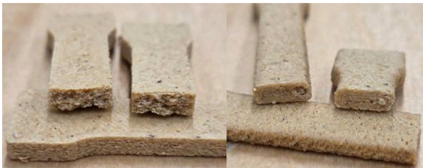
Figure 34. Test bars 3D-printed from PLA with 20% sawdust in a vertical (left) and horizontal (right) printing direction. (Image Tiina Marttinen)
