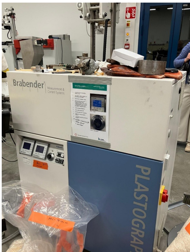
Figure 16. A laboratory-scale single-screw extruder for extrusion process evaluation. (Image Kirsti Cura)
