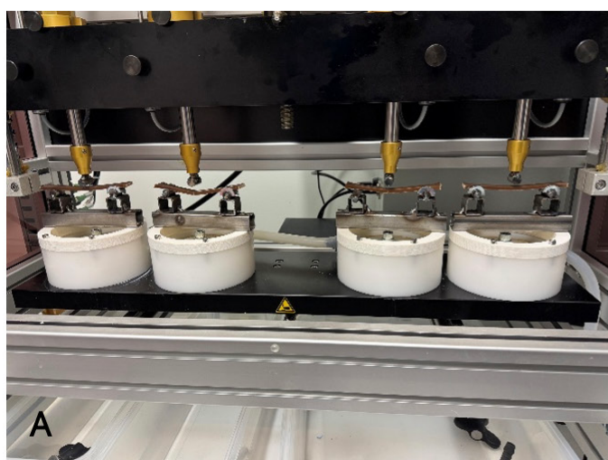
Fig. 47. A dental bending test simulator (A) was used to determine the survival of four identical samples in each group (B).
