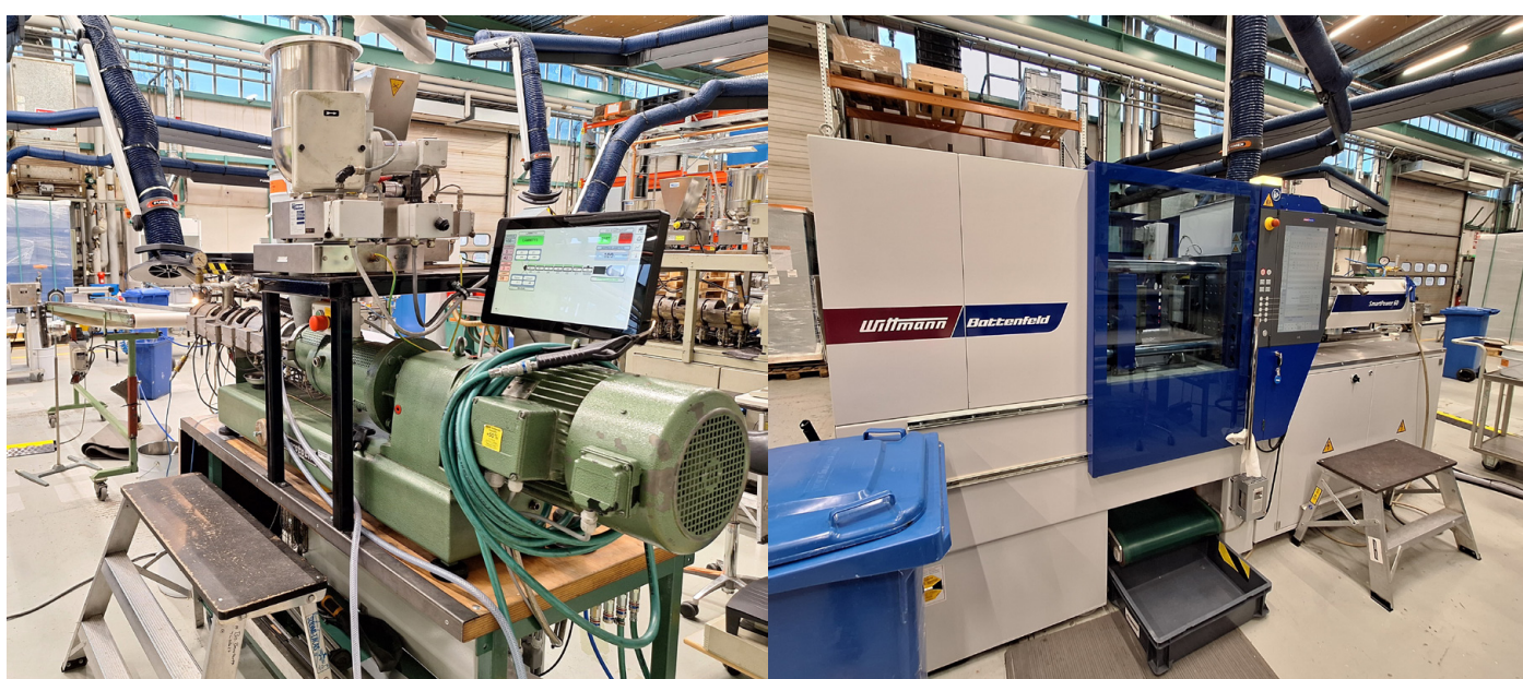
Figure 15. Compounder used for biocomposite compounding (left) and injection-moulding machine (right).
