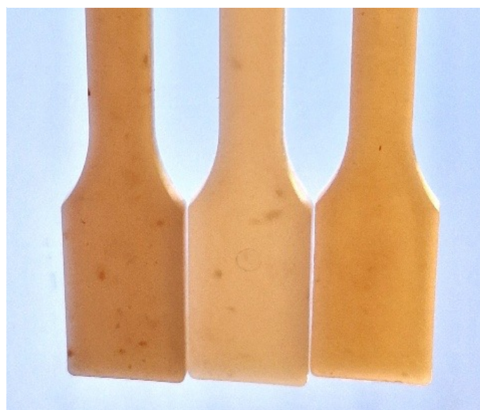
Figure 19. Injection-moulded bio-LDPE samples with 20% BSK fibres pre-treated in three different ways: compacting method, batch mixing, and foam forming.
