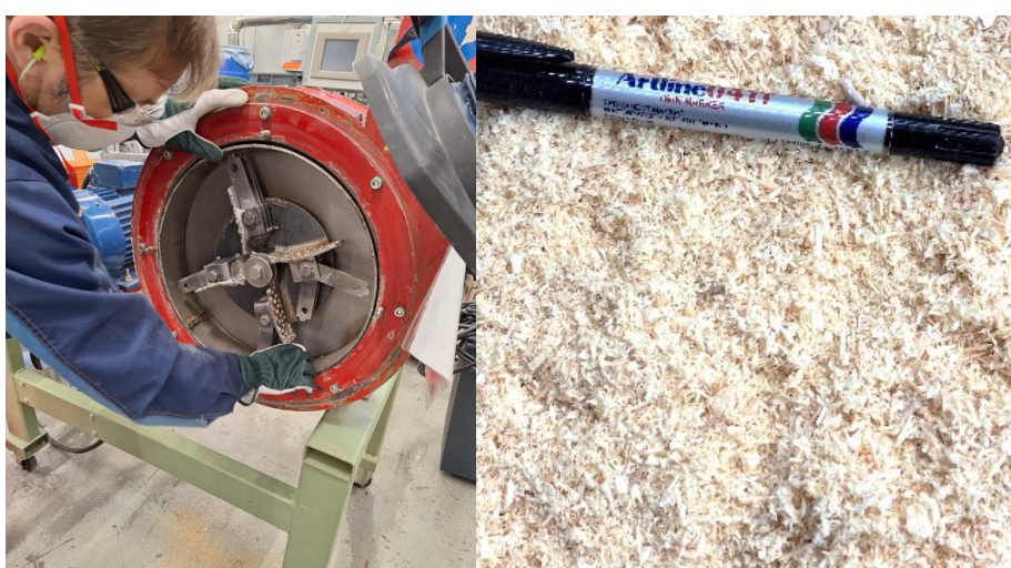
Figure 14. Rivakka hammer mill (left) and milled sawdust (right).
