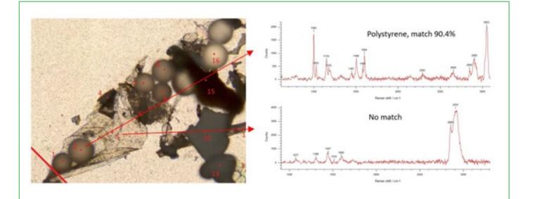
*Figure 21: Left: Particles extracted from sewage sludge for Raman analysis on a filter. Right: Examples of Raman spectra of the analysed particles.*
