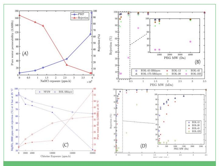
Figure 14: The effect of NaOCl exposure on: PWP and salt rejection (A); Retention of PEGs and PWPs of oxidised and LBL-coated membranes (B&D); Stability of 5 bilayer coated and commercial membrane NF270. (The Numbers denoted to the name of EOL membranes are the permeability of membranes).
