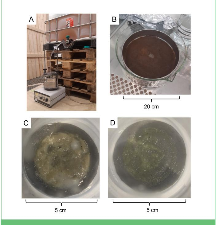
Figure 18: A) Filtration of 1 m3 of P&P effluent, B) the untreated sample representing solids (>20  $\mu$ m) from 1 m3 of P&P effluent, C) the solids (>20  $\mu$ m) from 250 L of P&P effluent after one H2O2 treatment, and D) the solids (>20  $\mu$ m) from 250 L of P&P effluent after two rounds of NaOH-Urea treatment in combination with H2O2 treatment.
