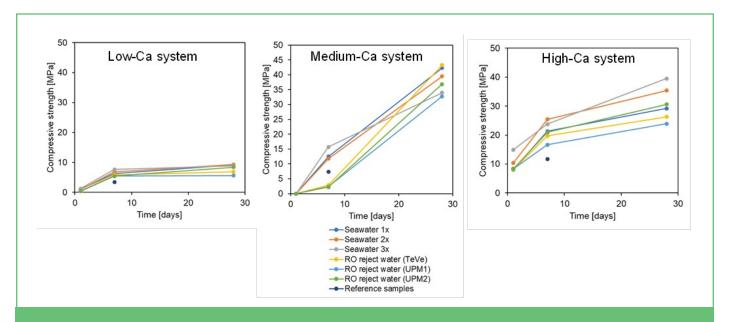
*Figure 13: Compressive strength of binders prepared with different high salinity waters using metakaolin (low-Ca system), mixture of metakaolin and blast furnace slag (medium-Ca system), and blast furnace slag (high-Ca system). Seawater 1x, 2x, and 3x refer synthetic seawater with 1x, 2x, or 3x salt content.*
