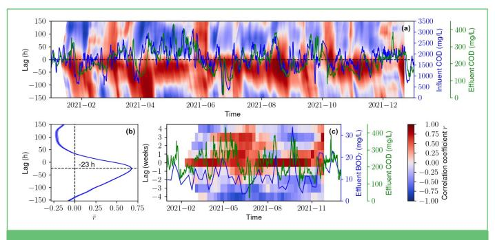
*Figure 9. (a) Time-dependent cross correlation (colour map) between the influent and effluent COD for different lags. (b) Average cross correlation for each lag. (c) As in (a) but for effluent COD and BOD.*
