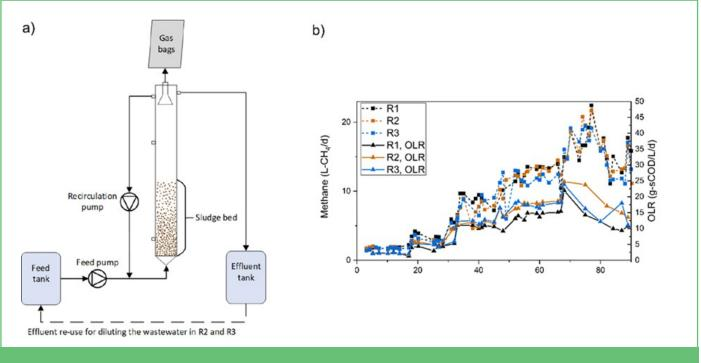
Figure 12: Process scheme (a) and methane production at different OLRs (b).
